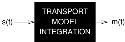
Figure 7.1 A representation of a black-box atmospheric-transport model, calculating \mathbf{m} = \mathbf{G}\mathbf{s} .
